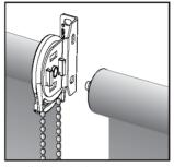
Note: If sharing a bracket between two shades, bracket can only be shared by a clutch and a pin end, not a clutch-to-clutch or
